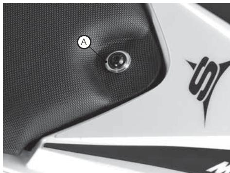
Remove the seat in direction **A** as shown in the picture.
