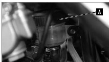
The rear brake fluid tank is located next to the mechanical start-up lever.
