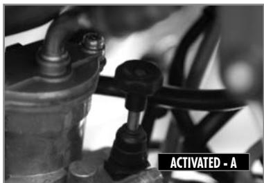
The choke is located to the right of the carburettor.
