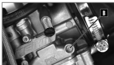
The carburettor is adjusted in-factory, but it may require small adjustments depending on the altitude and weather conditions.
