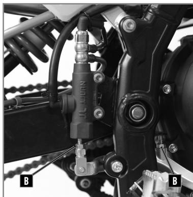
The rear brake is a hydraulic disc brake.
