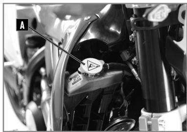
Follow the procedure listed below to check the fluid level. This operation must be performed with the engine cold:
