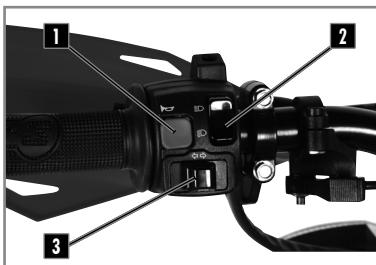
This switch is for the lights and other functions. It is positioned on the left side of the handlebar and has the following functions:
