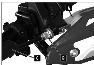
To adjust the clutch lever **A** lift the rubber cover **C** and use the adjusting fitting **B** to obtain a free play of 5mm.
