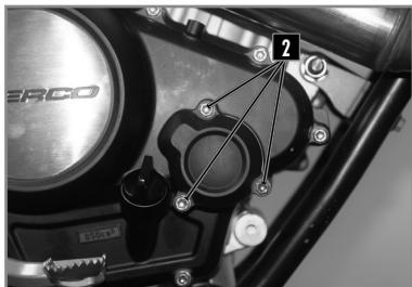
Remove the oil filter cover, on the right side of the engine, after having removed its three screws **2**.
