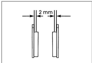
The condition of the brake pads can be checked by observing the end of the 2 pads on the caliper they should have a minimum thickness of 2 mm.
