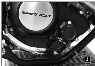
The oil level is checked with the dipstick attached to the filler cap on the right hand side of the motorbike **A**.
