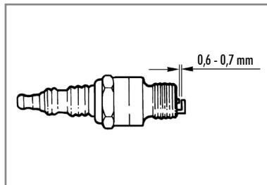
Keeping the spark plug in good condition helps to decrease fuel consumption and helps optimize the engine performance.
