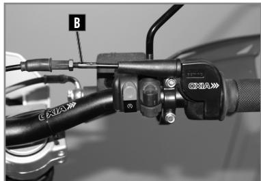
In the case where the throttle cable slack is greater than 3 mm, measured from the edge of the handle, it is necessary to perform an adjustment using the cable adjuster **B**.
