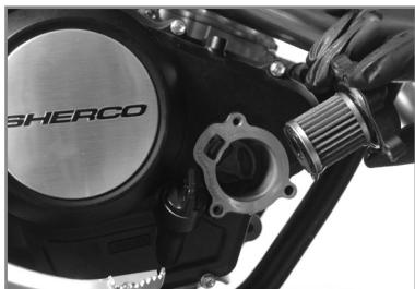
Replace the oil filter, making sure that it is fitted in the right direction: the filter cover pin must enter the filter through its open side.
