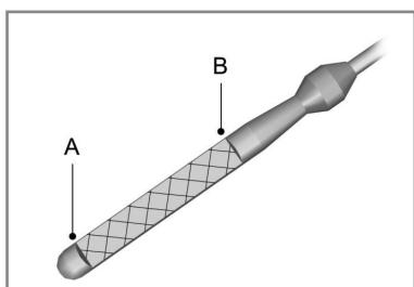
The oil level must be between the MIN **A** and MAXI **B** marks.
