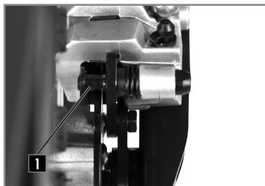
The state of wear of the brake pads can be checked by observing the end of the 2 pads on the caliper 1 they should have a minimum thickness of 2 mm.
