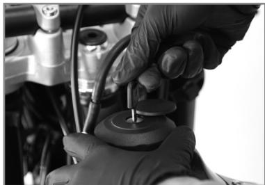
To open the fuel filler cap, insert the key into the lock and turn it counter-clockwise, then turn the cap in the same direction.
