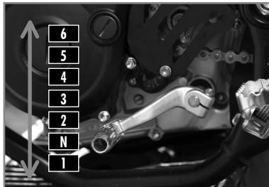
The gear shift lever is mounted on the left side of the engine.
