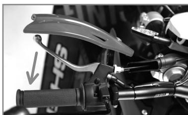
Pull the clutch lever and press the starter button 1. Starting the engine is possible with a gear engaged, unless the side stand is extended.
