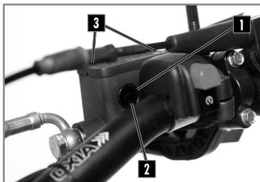
Check for the presence of brake fluid through the sight glass **1**.
