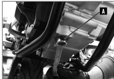
This operation must be carried out with the engine warm. Keep the motorbike in an upright position with respect to the ground. Place a container under the motorbike to collect the used oil.
