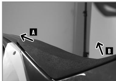
Remove the seat in direction **A** as shown in the picture.
