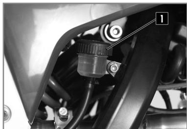
The minimum brake fluid level should never be below the [MIN] mark on the brake fluid reservoir.
