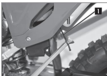
Remove the rubber safety latch 1, using your foot on the shaft unfold it until it supports the weight of the bike.
