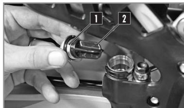
Remove the cap **1** with its membrane **2**.
