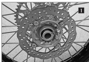
Check if the brake disc is not dirty or contaminated with oil or grease.
