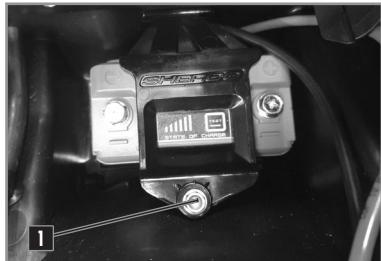
The battery is located at the bottom of the filter housing.
