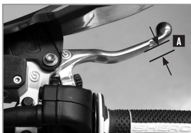
Pull the lever toward the handlebar and check the free play **A**.
