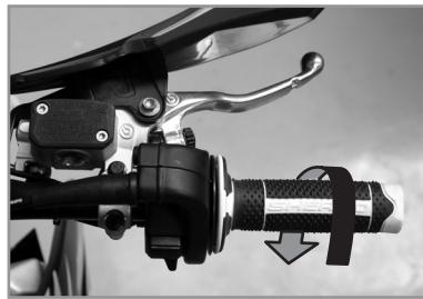
With the handlebars facing straight ahead, check that the throttle twist grip functions properly.
