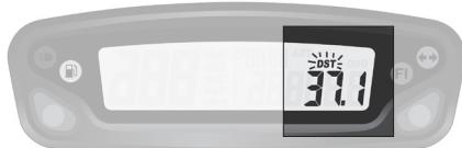
Fig 6 Adjustable trip distance function
