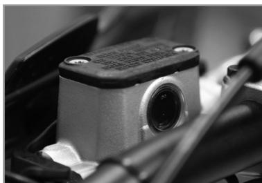
Make sure that the reservoir is in a horizontal position. Check the fluid level through the sight glass.
