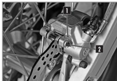
Check if the brake discs are not contaminated with oil or grease. In they are, clean the discs with brake cleaner.
