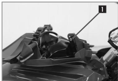
The headlight beam is adjusted with the motorcycle in running order with its driver seated on the saddle. To set headlight beam, loosen screw 1.
