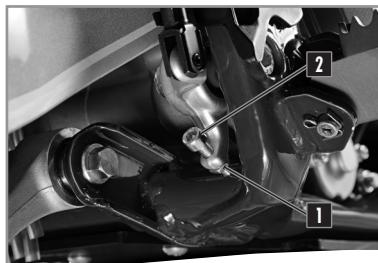
The position of the brake pedal can be adjusted as follows: loosen the lock nut 1, loosen or tighten the screw 2 to obtain the desired position.
