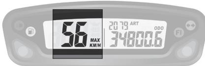
**Fig 2 MAX speed function**
