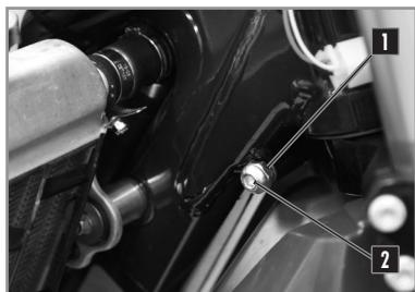
The steering angle can be changed using the set screws located on the bottom of the steering column. Loosen the nut **1** and tighten the screw **2** until you have the steering angle desired. Tighten the nut and do the same operation on the other side.
