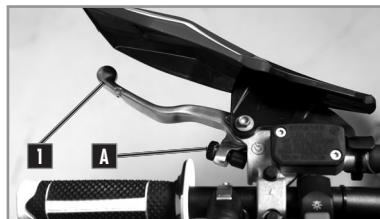
The clutch lever **1** is on the left handlebar and has an adjustment screw **A**.
