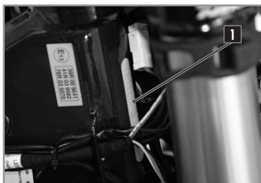
**1** The serial number of the vehicle is stamped on the right side of the steering tube.
