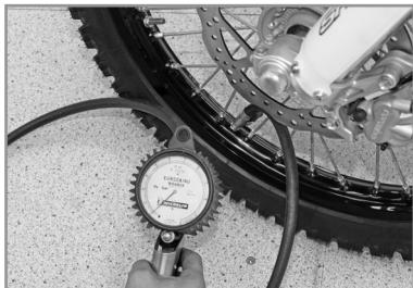
Regularly check the tire pressure with a precision pressure gauge.
