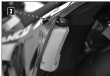
Check the fluid level in the expansion container.
