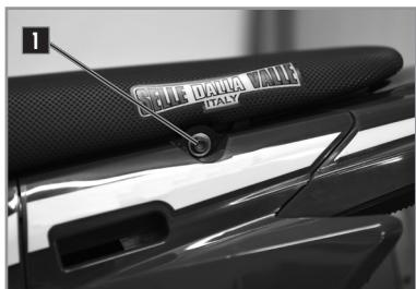
Unscrew the fixing screw 1 on each side of the seat.
