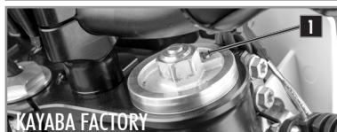
After some time of operation, the air accumulates under pressure in the fork.
