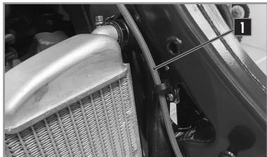
Ensure proper routing of cables and hoses 1.
