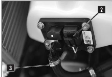
Check the adjustment of the radiator guards in relationship to the fuel tank.
