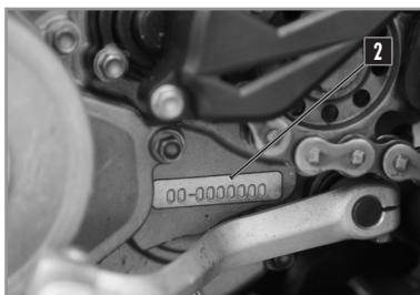
**2** The engine serial number is stamped on the left side of the engine housing.
