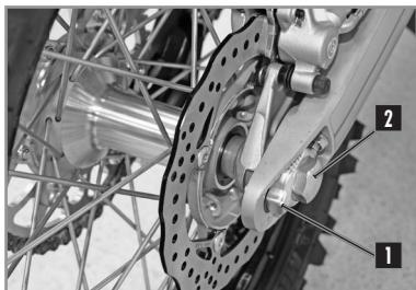
Install the chain tensioner **1** and install the nut **2** but do not tighten.
