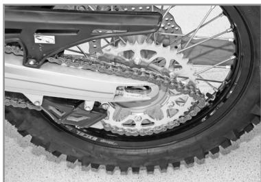
Install the rear wheel in the swing arm and install the axle (grease the axle prior to installation).
