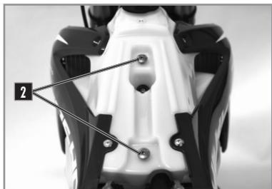
Replace the seat, ensuring that it is correctly fitted into the tank pads 2.
