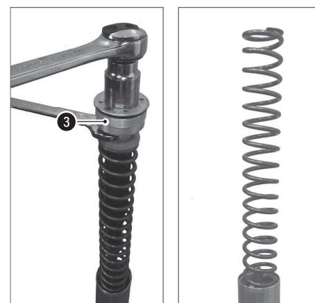
Loosen the **preload adjuster** ③.
